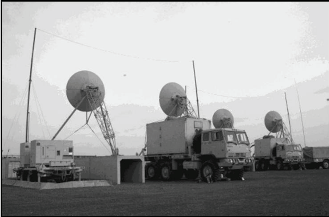
Figure B-10. AN/TRC-170(V)2 Heavy TROPO
